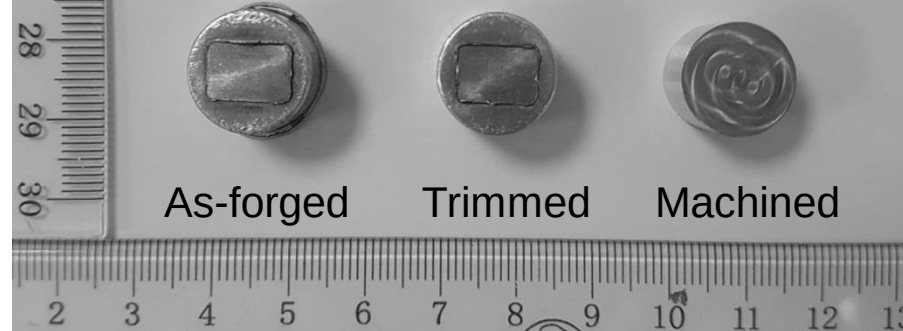
Figure 12. Top, side and bottom view images of the KYO-forged, KYO-trimmed and post-machining parts arranged in the order of part shape evolution.
